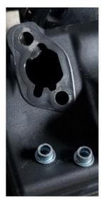
Re-install airbox with barrel nuts use washers if necessary. Re-connect hose
