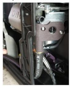
Optional: For quick switching between gasoline and alt fuels, install a lock off valve here. Sold seperately
