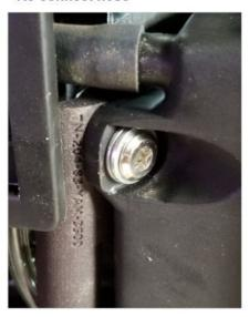
Re-use bottom airbox bolt. Use bushing for spacer with loctite
