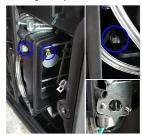
Push hose onto barb (use hose clamp if necessary). Install adapter and route hose as shown
